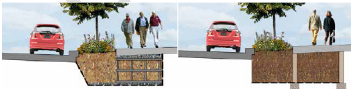
Figure 2-3 Stormwater tree well filter conceptual examples: modular suspended pavement system (left), column suspended pavement system (right). (Courtesy of Philadelphia Water Department)
