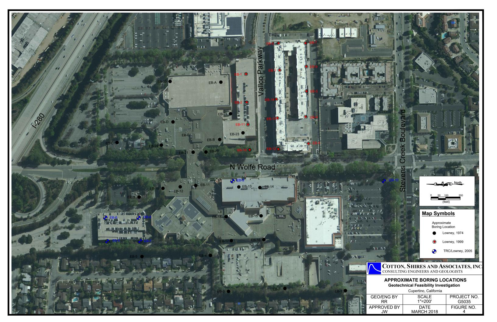
interpret this difference between the older investigations and the newer investigations to be the result of the Vallco development where excavation/compaction of the loose upper soils was performed. The recent borings reveal that, in general, the site is underlain by medium dense to dense sands, and stiff to hard clays.
