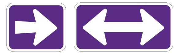
Arrow signs are 12"w x 10"h, and 20"w x 10"h, per spec. Arrows are 7.5 inches high. Digital print on 3M EG reflective vinyl, coated with 1160 Graffiti film and mounted to .080 aluminum sign blanks.
