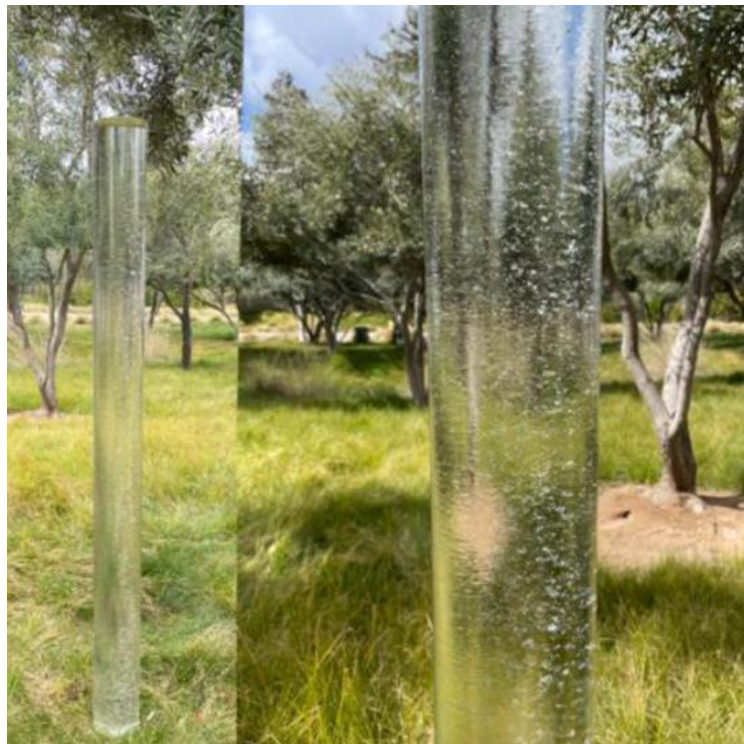
Figure 5: Sample glass cylinder demonstrating translucence and variation due to materials and the manufacturing processes
