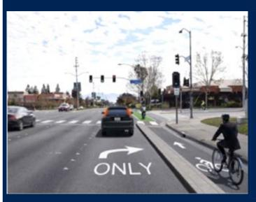
The next Phase of the SCB CI IV bikeway, from Wolfe Road to US-85. Design includes signal improvements and a concrete island separating vehicles from bicyclists.
