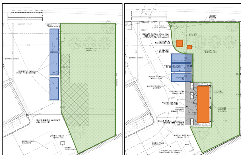
Figure 3: Hydrogen equipment (orange), parking (blue), and landscaping (green) on the eastern end of the property: existing approved conditions (L) and proposed site plan (R).
