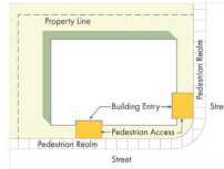
Figure 2-2 Orientation of building on corner lot.
