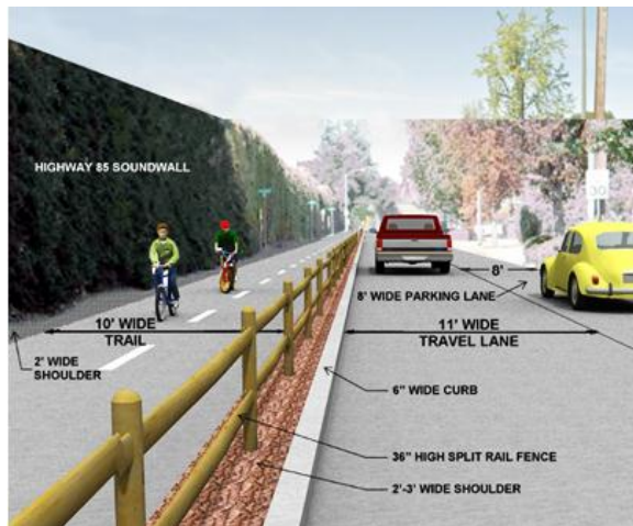
Figure 3 – Potential Configuration on Bernardo Avenue, between Astoria Drive and The Dalles Avenues
