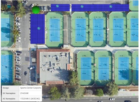
This property allows for the PV system to be well-aligned to west and south-facing solar access. The arrays are situated to ensure they do not interfere with vehicular traffic, and to minimize impacts to the tree in the corner between the two arrays. This tree would need to be slightly trimmed to ensure maximum solar access. The small trees under the northern arrays would need to be removed.
