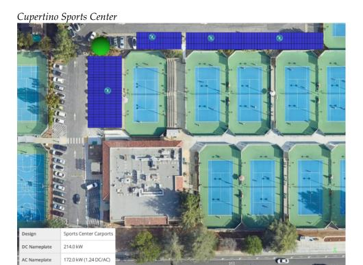
This system is well-aligned to the west and south-facing solar access. The northern array is split around north-south site access path to allow for any traffic which could interfere with the carport array.
