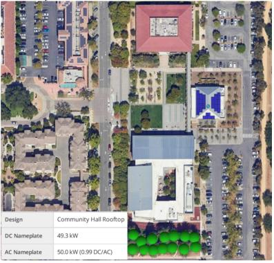
This is an ideally oriented system with rooftop racking. Roof penetrations will not be required, as the system will be able to clamp to the existing standing seam roof profile.
