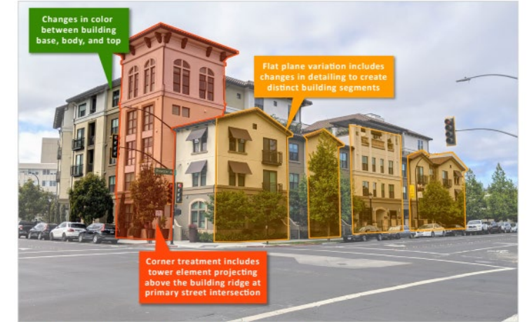
Figure 29: Examples of massing breaks in mid-rise buildings (Section 4.1.6.C)
