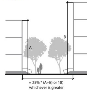
Figure 2: Minimum Width for Pedestrian Access
