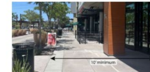
Minimum 10' paved walkway at ground floor commercial between face of building and edge of walkway.
