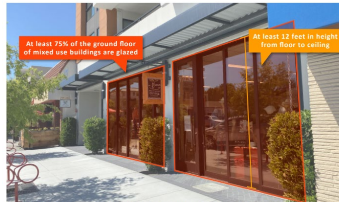
Figure 33: Ground floor commercial uses shall be at least 12 feet in height. (Section 4.2.1.B)
