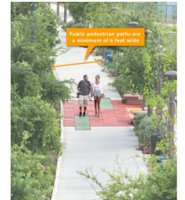
Figure 11: Public pedestrian paths shall be a minimum of six (6) feet wide. (Section: 3.1.1.A)
