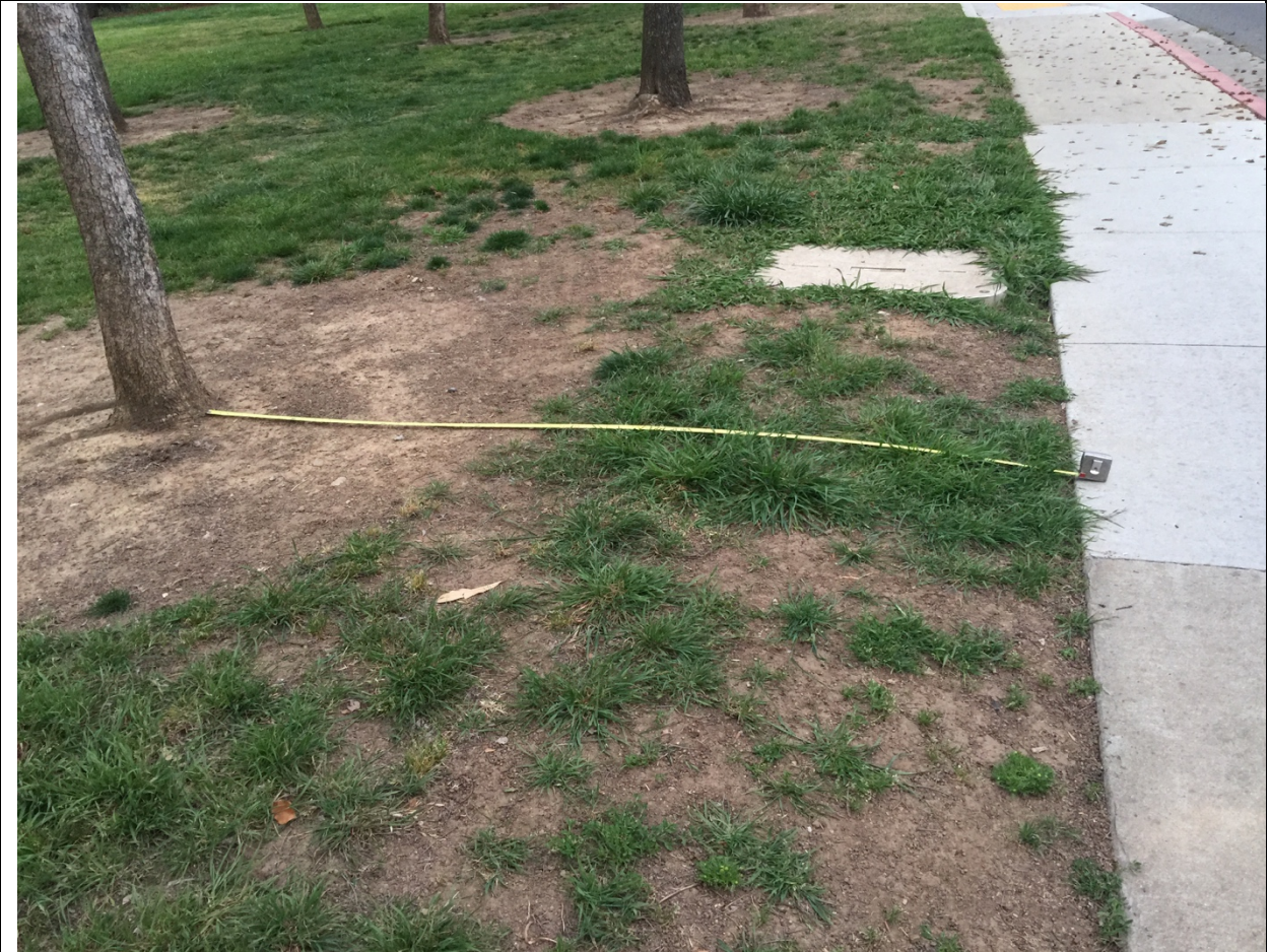
Attachment B, distance from tree trunks to sidewalk is about 7-8 feet. Note the bend of the tape measure indicates raised elevation of the open ground relative to the sidewalk.
