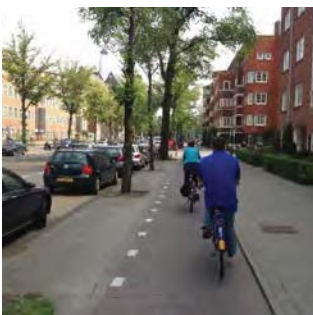
Figure 4.8. Raised cycle tracks eliminate conflicts between vehicles parking and loading and people on bikes. Image source: "Sustainable Transportation in the Netherlands"
