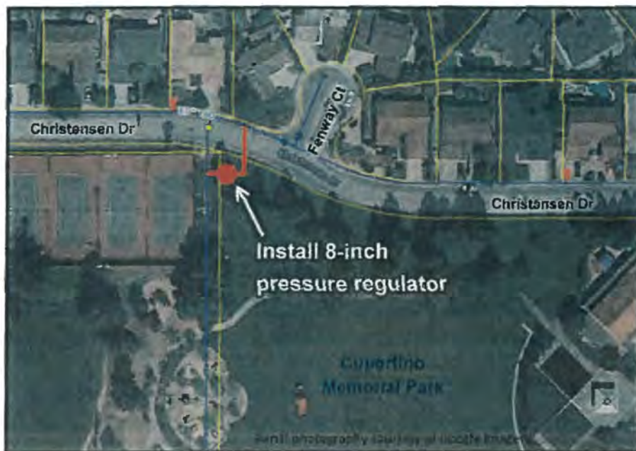
Figure ES-3. Recommended 8-inch Pressure Regulator Installation
