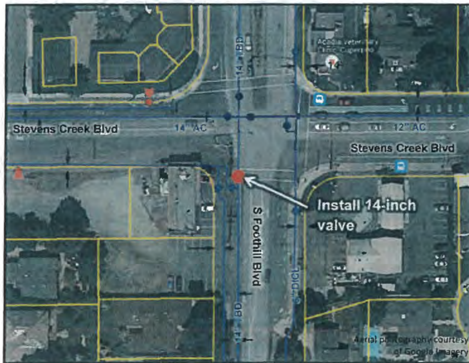
Figure 15. Recommended 14-inch Valve Installation
