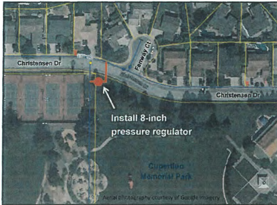
Figure 14. Recommended 8-inch Pressure Regulator and Immediate Vicinity
