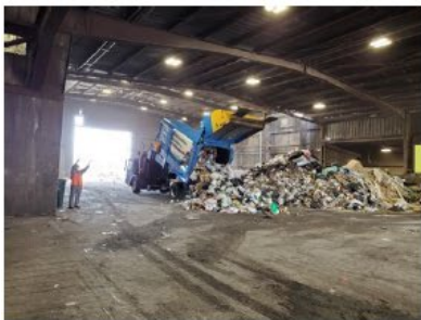
Step 1 Select sample from tipped load
